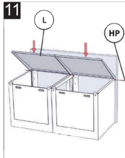
Attach lids to the unit with hinge pins. Align pins with holes and tap into place with a mallet.
