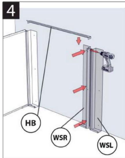
Now insert the other wall fixing strips onto the tabs of the corner and straight brackets.
