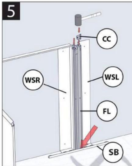
Insert the filler between the panels and slide into the straight bracket, ensuring slots at top of filler are in line with slots at top of wall fixing strips. Place the plastic caps into the wall fixing strips to join them to the filler.
