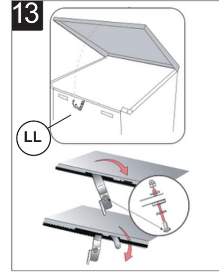
Attach the latch to the door using the supplied screw/washer/nut as per above. Rotate the Latch clockwise to 'lock' into the top lid.
