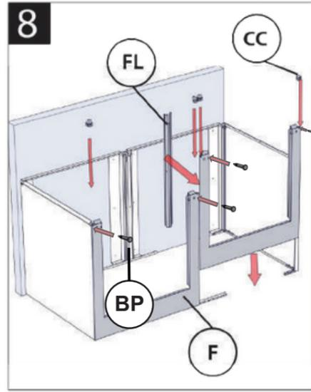
Slide the front panels into position and insert the filler and caps. Insert 4 x BP into slots on the front panels through the corner caps.
