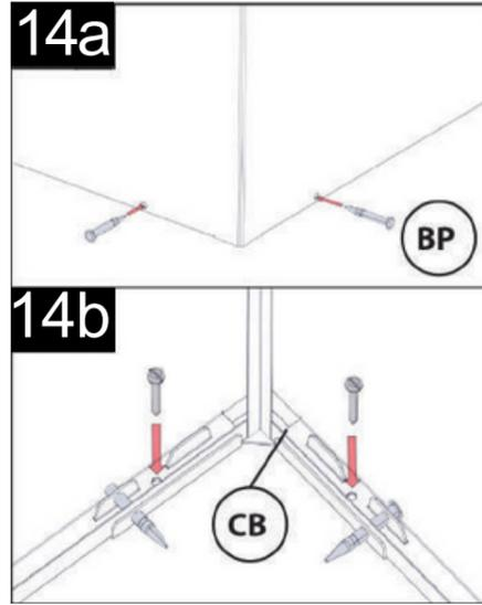
Push base pins into holes in the bottom edge of outer panels and through corner bracket (a). Anchor box to timber base frame as shown or concrete slab / other flat surface (b). Do this for for all 4 corners.
