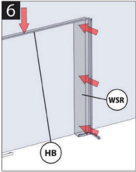
Slide the wall strip onto the corner bracket and attach to wall using appropriate fixings.
