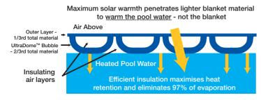
As the above illustration demonstrates, the air in the bubbles, and the air trapped between the top layer of the blanket and the water - between the bubbles - effectively form a thick layer of insulation across the entire blanket area.
