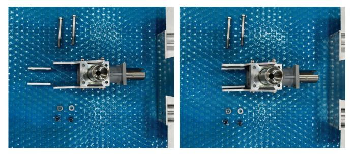
Mount the gearbox to the post and tighten all mounting bolts.
