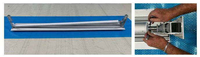
**10.** Lift the slave end and insert into the tube. Insert the mounting bolt then tighten.
