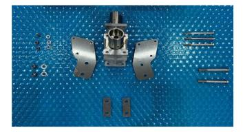
Install the large mounting plate onto the gearbox using 3 x 6mm bolts, taking note of the plate offset.
