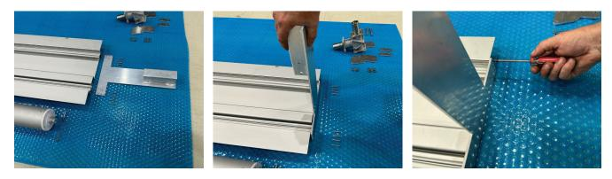
**4.** Decide what end you want the gearbox winder to be installed. Lay out all parts and note the slotted coupling required for handle operation is to be at the top.
