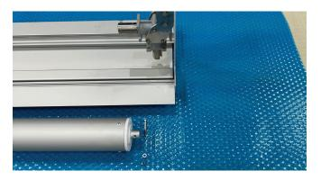
8. Prepare the slave end ensuring the flat side of the plastic mounts to the frame and the extended side to the tube – then slide the mount onto the end slug.
