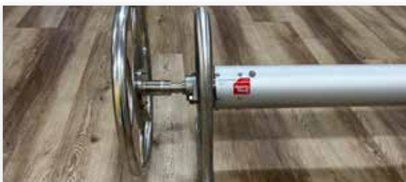
17.2. Slide handwheel onto end slug shalf.
