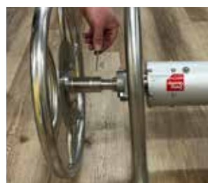
18.1. Use bolt to secure handwheel.
