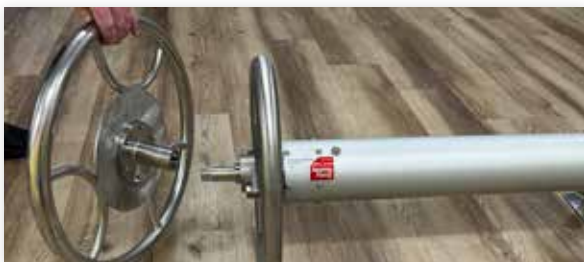
17.1. Line up handwheel to the square drive.
