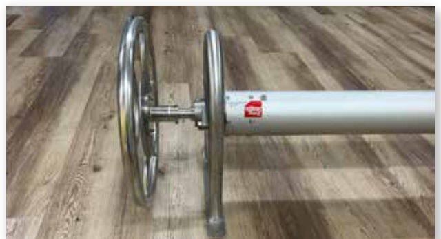
18.1. Use bolt to secure handwheel.
