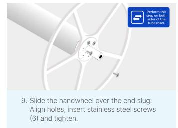
Note: for UTC 4 spoke hand wheels, clip the handwheel into the end slug then secure with the 3 stainless steel screws and tighten.
