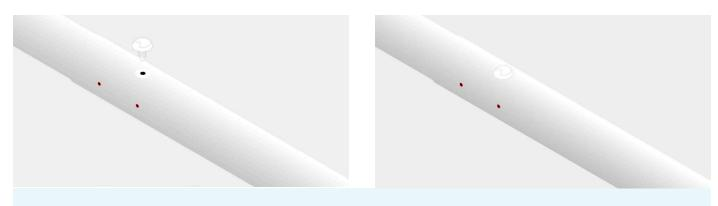
3. Place the white feather plugs into the white marked holes to keep tubes in place prior to drilling self drilling screws. To make a custom size length, use the 6.5mm drill bit supplied to drill new feather plug holes.
