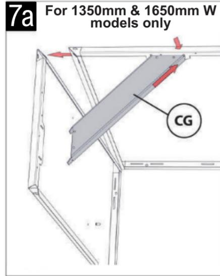
Insert corner gussets into the side and front panels by inserting into the corner and pushing downwards.
