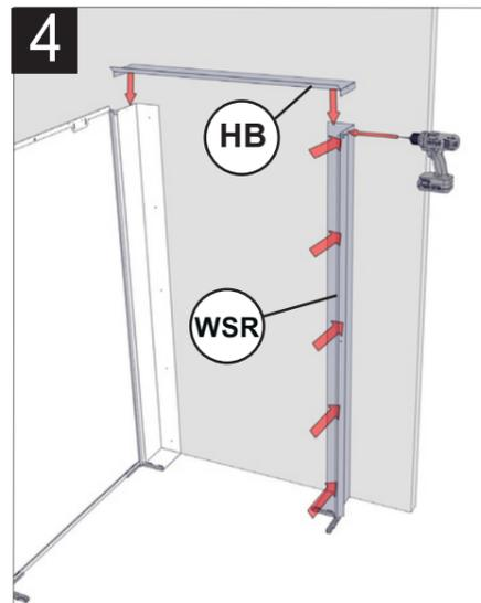
Install the Horizontal Bridge Cover, installed on the outside of the wall fixings strips. Use 2 metal tek screws to attach the horizontal bridge cover to the wall fixings strips. Fix the wall fixing strips to the wall using appropriate wall fixing anchors through the pre drilled holes.
