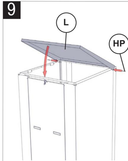
Attach top door to unit with hinge pins. Align pins with holes and tap into place with a mallet.
