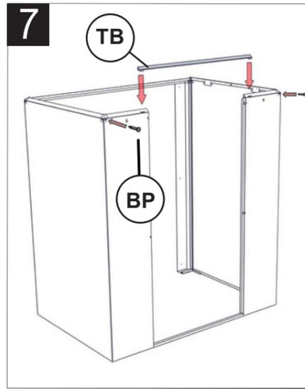
Insert Top Brace into slots in Front Left and Front Right Panels. Insert 2 x BP into slots on the front panel through the corner caps.
