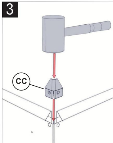
Now insert a plastic cap into the holes in the top of the panel to join them. Tap into place with a mallet.
