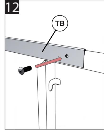
Secure Top Brace to Front Left and Front Right Panels with a Tek Screw.
