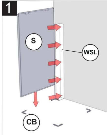
Locate slots on bottom of side panel and wall fixing strip and push down onto corner bracket. Fix wall fixing strip to wall using appropriate anchors.
