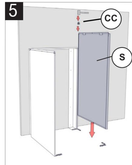
Align the slots in the side panel and slide into position. Insert the cap.
