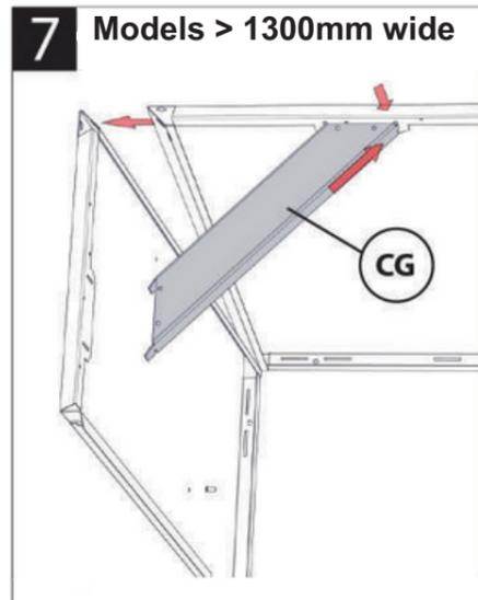
**7 Models > 1300mm wide** Insert corner gussets into the side and front AND side and rear by inserting into the corner and pushing downwards.
