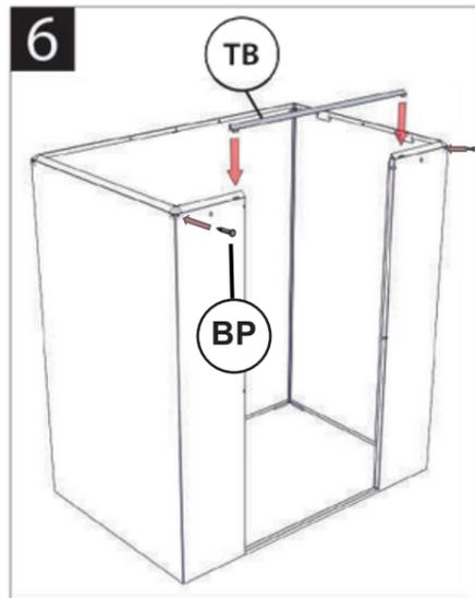
**6** Insert Top Brace into slots in Front Left and Front Right Panels. Insert 2 x BP into slots on the front panel through the corner caps.
