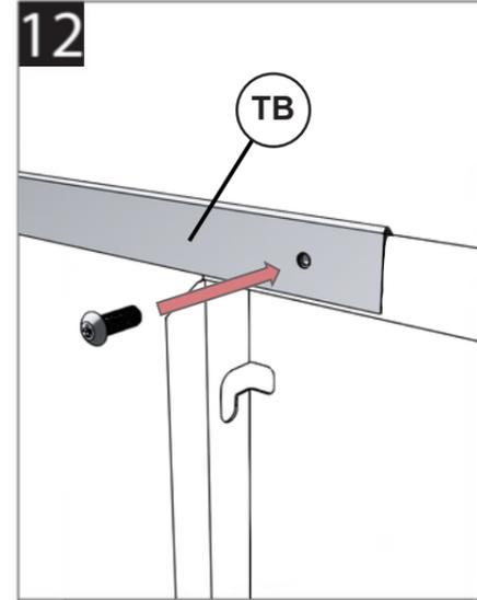
**12** Secure Top Brace to Front Left and Front Right Panels with a Tek Screw.
