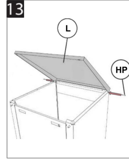
**13** Attach top door to unit with hinge pins. Align pins with holes and tap into place with a mallet.
