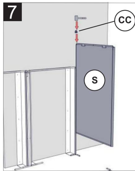
Slide the side panels into position and insert the filler and caps.
