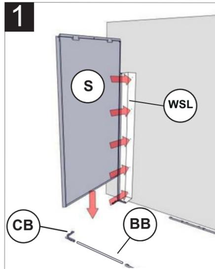
Locate slots on bottom of side panel and wall fixing strip and push down onto corner bracket. Fix wall fixing strip to wall using appropriate anchors.
