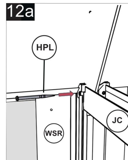
For the central join, tap the centre hinge pin through both top door and corner caps.
