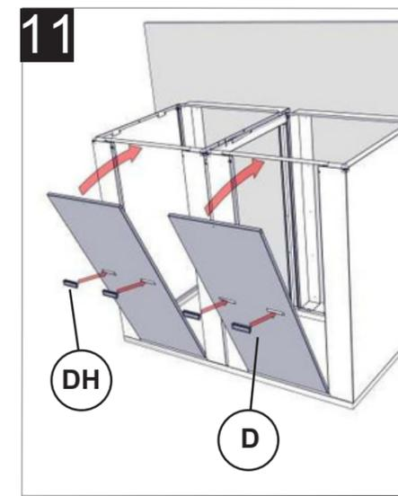
Insert the handles into the door until a "click" is heard. Place the removable front door into the panel by placing the lip of the door over the front panel step. Insert the door by aligning the studs on the side with the slots in the front panel. Push in slightly and then down.
