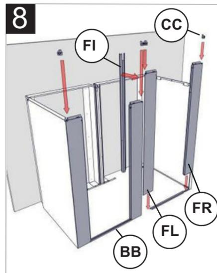
Slide the front panels into position in the bottom brace and insert the filler and caps.
