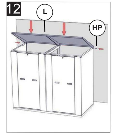
Attach lids to the unit with hinge pins. Align pins with holes and tap into place with a mallet.
