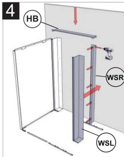
Now insert the other wall fixing strips onto the tabs of the corner and straight brackets. Screw horizontal bridge cover into Left and Right Wall Strips.
