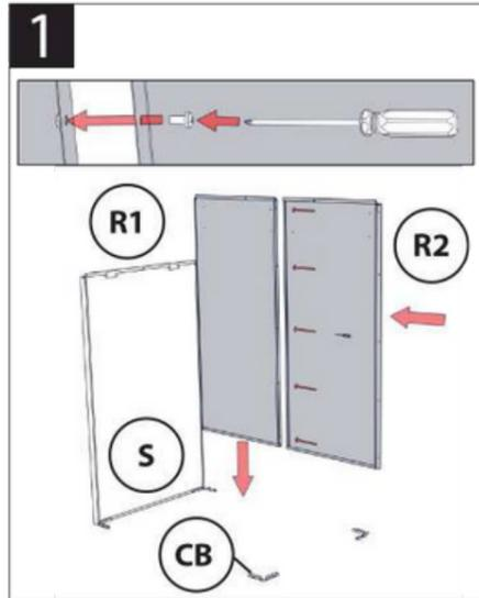
Screw Rear Left and Rear Right panels together using M5 screw as shown. Push down onto corner brackets with the Side Panel.
