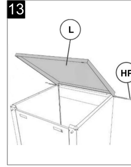
13 Attach top door to unit with hinge pins. Align pins with holes and tap into place with a mallet.
