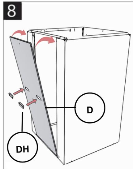
8 Insert the handles into the door until a "click" is heard. Place the removable front door into the panel by placing the lip of the door over the front panel step. Insert the door by aligning the studs on the side with the slots in the front panel. Push in slightly and then down.
