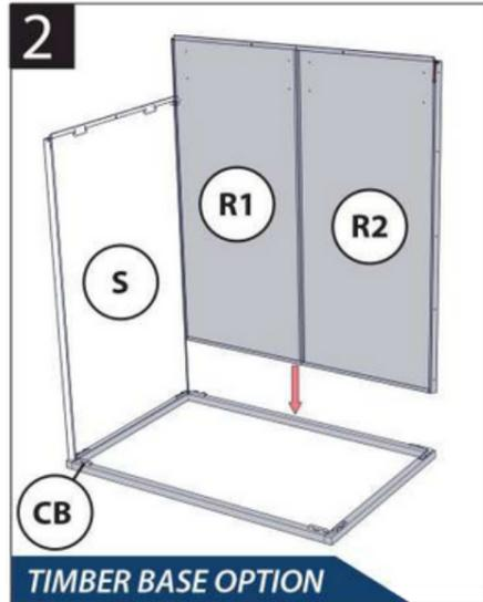
If no concrete slab / other flat surface is available, use timber base frame as shown.
