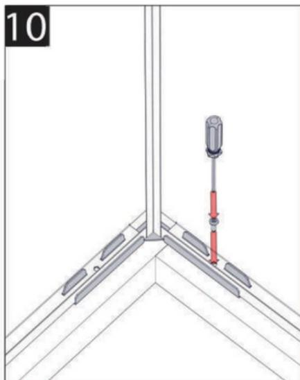
10 Anchor box to timber frame as shown or concrete slab / other flat surface.
