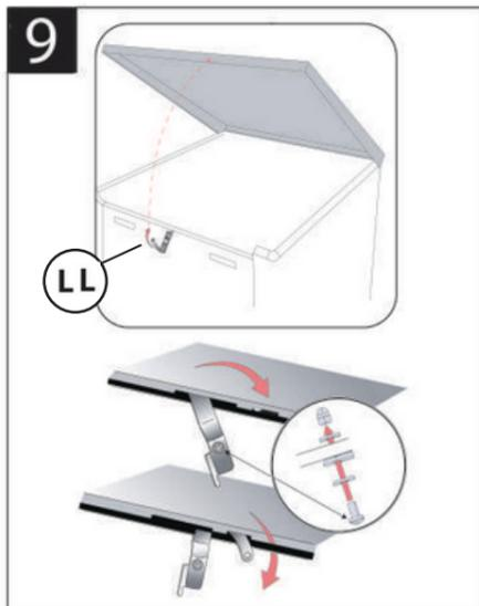
9 Attach the latch to the door using the supplied screw/washer/nut as per above. Rotate the Latch clockwise to 'lock' into the top lid.
