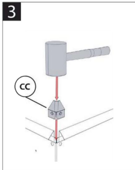
Now insert a corner cap into the holes in the top of the panel to join them. Tap into place with a mallet.
