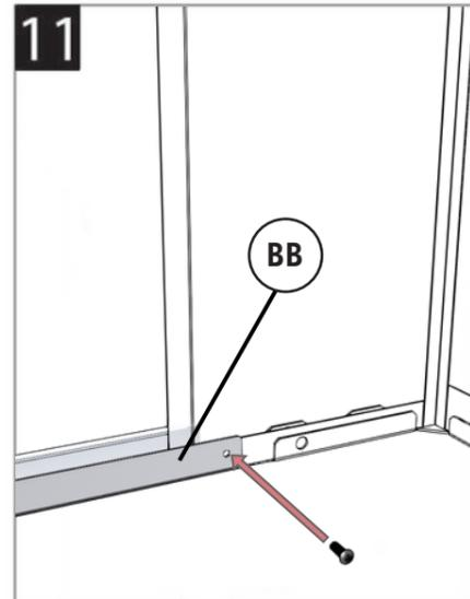
11 Secure Bottom Brace to Front Left and Front Right Panels with a Tek Screw.
