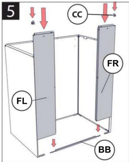
Slot Front Left and Front Right panels into the Lower Brace and Corner Brackets. Tap Corner Caps into place with a mallet.
