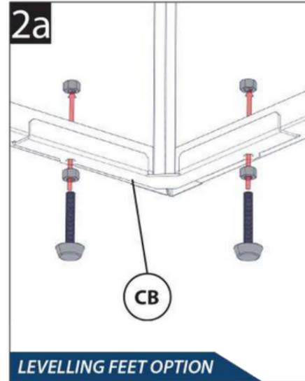
If installing on an uneven / unlevelled surface, please use the optional feet (through holes in bottom corners) to raise the box and adjust the nuts below / above the corner bracket to suit.
