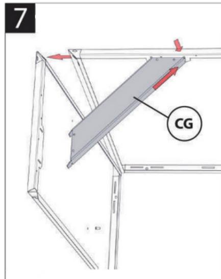
7 Insert corner gussets into the side and front AND side and rear panels by inserting into the corner and pushing downwards.
